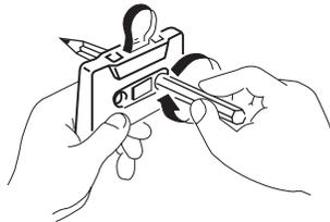
**Caution:** If you do not remove the excess slack, the tape could become tangled in the record/playback mechanism.
