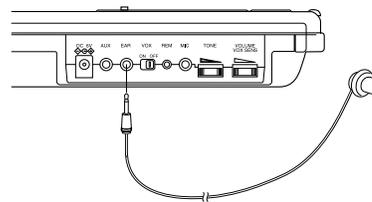
**Note:** Connecting the earphone automatically disconnects the built-in speaker.
