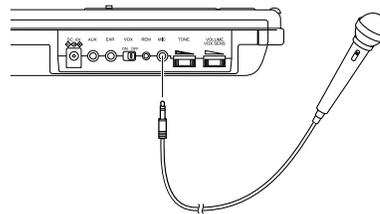
**Note:** If the external microphone has a separate, smaller plug for remote operation, insert that plug into the **REM** jack. Then you can use the microphone's remote switch to stop or start the recorder.
