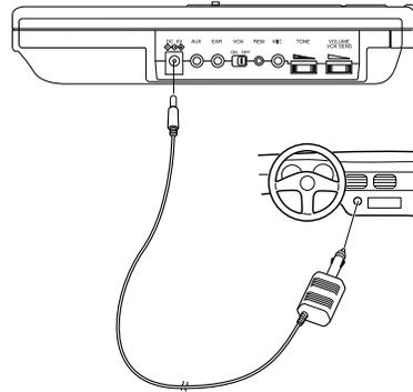
1. Set the DC adapter's voltage switch to 6V.
