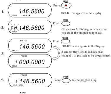
Note: Press to escape from programming mode before step 4. **Example 2: Programming from SEARCH mode.**
