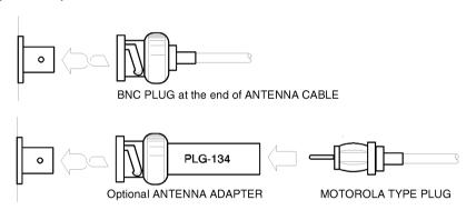
Connect your Antenna plug here. If you have a Motorola-type plug, use the optional adapter ( PLG 134).
