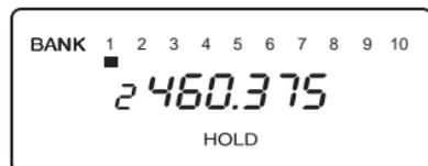
**Note:** To clear a mistake while entering the frequency, press **E** twice, and start over.
