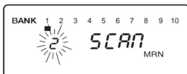
When an active channel is displayed, the scanner will alternate between the frequency and the Marine channel number. For example, 156.800 alternates with CH 16.
