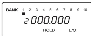
*Channels with no frequencies are automatically locked out.*
