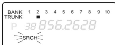
**Note:** You will see the frequencies quickly displaying as your scanner looks for the data channel which controls the system.
