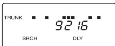
**Note:** If more than 20 channels are stored in a bank, then the indicators represent multiple channels. For example, if 29 channels are programmed, the first 9 activity indicators each represent two channels.
