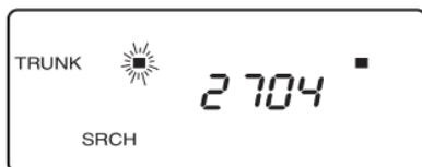
*The ID is locked out, and the next active ID displays. You can lockout up to 100 IDs.*
