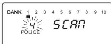
**Note:** *You can lockout up to 20 frequencies in SVC Scan mode. The 21st locked out frequency entered causes the first locked out frequency to unlock.*
