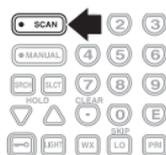
2. The indicator for each bank which will be scanned appears in the display, while the bank being currently monitored flashes. You can deselect banks from active scanning by pressing their number on your keypad. The indicator for each deselected bank turns off, and the bank's channels are not scanned.
