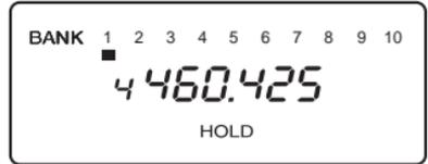
3. Press and hold **PRI** for two seconds to designate this channel as your new Priority Channel.
