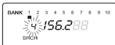
When data skip is active, your scanner may pause momentarily on an unwanted signal but will resume searching in 2 or 3 seconds. Data Skip does not function when the **AIR** Band is selected.
