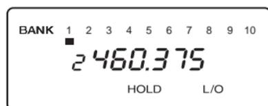
3. Press **(L/O)** to unlock the channel.
