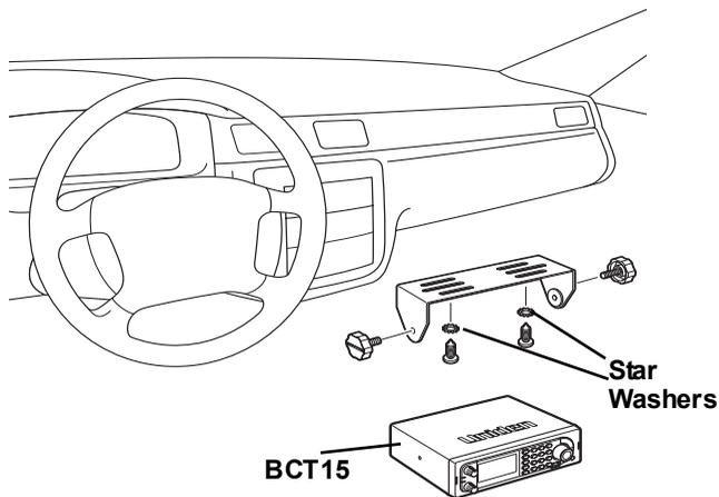
1. Using appropriate screws or other hardware, secure the bracket.
