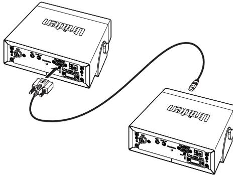
1. Plug the smaller end of the included connection cable into the Front Port. Then connect the DB9 end of the cable into the Rear Port. Be sure to set the scanner using the Front Port to **Front** and the other unit to **Rear** when making the speed selection.
