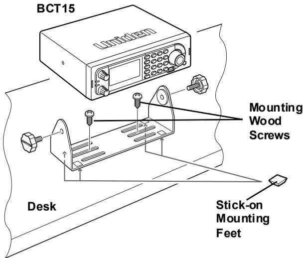
To secure the radio, by means of the mounting bracket, to a surface, follow the steps below:
