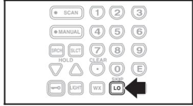
**Note:** You can program 10 skip frequencies. The 11th skip frequency entered causes the 1st skip frequency to unlock.
