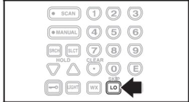
3. The scanner immediately resumes scanning because the locked out channel is no longer in the scanning sequence.
