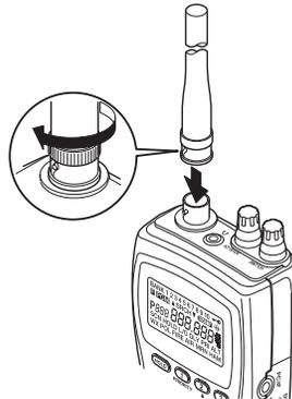
To attach the supplied flexible antenna to the connector on the top of your scanner, align the slots around the antenna's connector with the tabs on the scanner's BNC connector. Then slide the antenna's connector down over the scanner's connector and rotate the antenna connector's outer ring clockwise until it locks into place.
