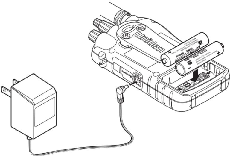
You can power your scanner using two alkaline, or rechargeable AA batteries.
