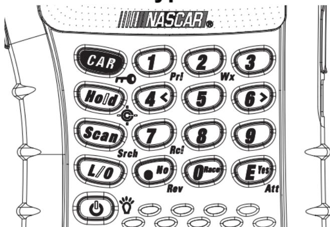
Your scanner's keys have various functions labeled on the key tops and below the keys. To select the function labeled on a key, simply press the key. To select the function labeled below a key, hold down **[Func]** on the left side of the scanner then press the key. **F** appears on the display.
