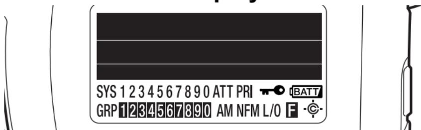
The display has indicators that show the scanner's current operating status. The display information helps you understand how your scanner operates. The dark area shown above the icons in this illustration is the text display area. Information about the currently tuned frequency appears here.
