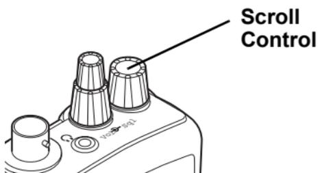
Turn the scroll control on top of the scanner to select a channel or frequency in Hold mode, select menu items in Menu mode, and to select a character while editing a name. You can also press the scroll control down instead of pressing **E** on the keypad to select an item.
