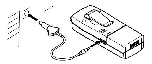
**Note:** If you installed rechargeable nickel-cadmium batteries in the scanner, connect the DC adapter to the CHARGE jack instead of the POWER jack. This lets you use the DC adapter to power the scanner and recharge the batteries at the same time.
