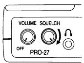
3. Turn VOLUME/OFF clockwise to set the scanner's volume about half way.
