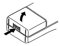
3. Remove the batteries from the battery compartment and the cover (if necessary).
