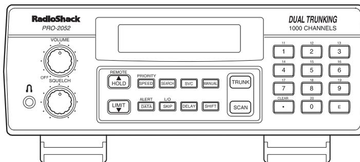
**VOLUME** Turns the scanner on or off and adjusts the volume.
