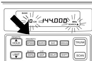
**Note:** You can use HyperSearch only in the 5 kHz step bands (29–54 MHz, 137–174 MHz, and 216–224.995 MHz).
