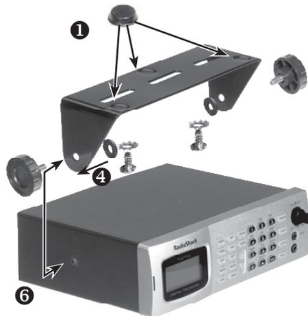
2. Use the supplied mounting bracket as a template to mark positions for the two mounting screws.
