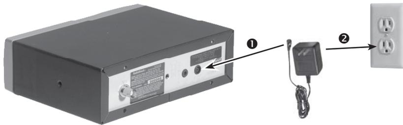
1. Connect the tip of the supplied AC adapter to the DC 13.8V jack at the rear of your scanner.
