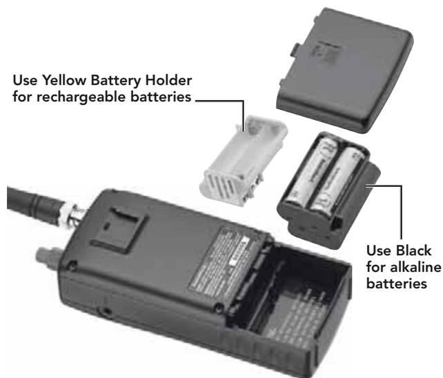
**Warning:** Never install non-rechargeable batteries in the yellow rechargeable battery holder. Non-rechargeable batteries can get hot or explode if you try to recharge them.
