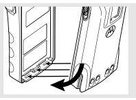
2 Press the top of the battery against the radio until both latches click into place.
