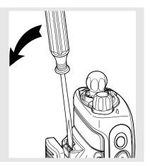
2 Slide the belt clip upward to remove it.
