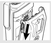
**2** Pull the top of the battery away from the radio.
