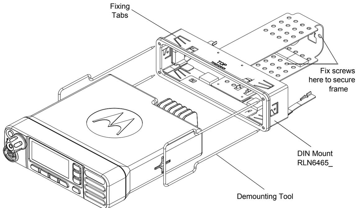
**Figure 2-10 Dashboard Mounting for MOTOTRBO XPR 5000 Series**
