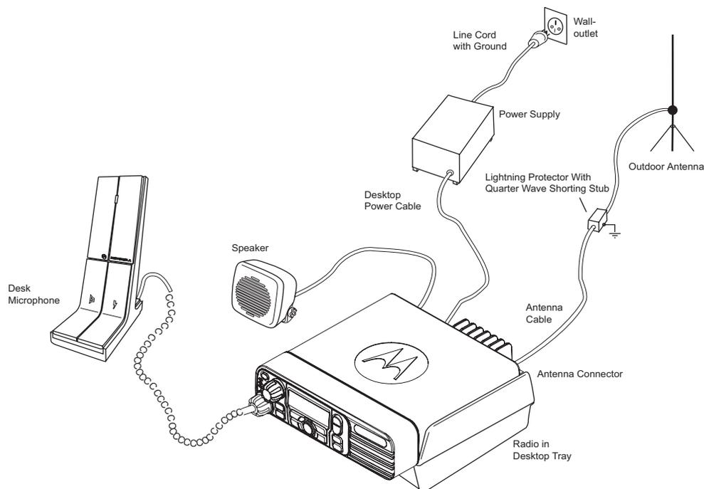
**Figure 1-7** Example of a Base/Control Station Configuration
