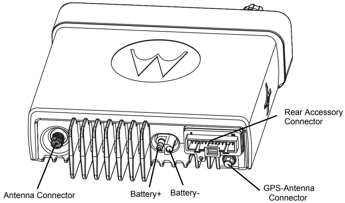
**Figure 1-5** Back View of the Mobile Radio
