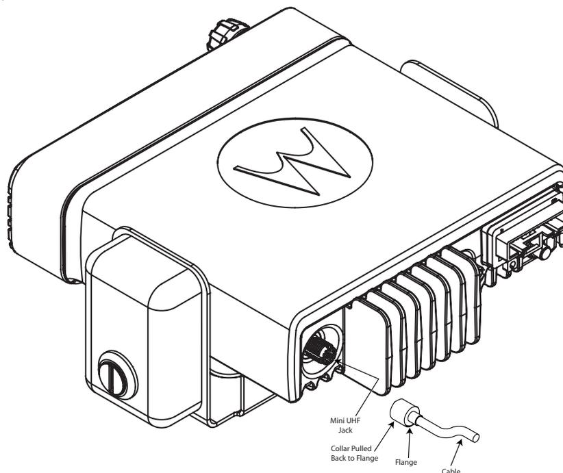
**Figure 2-14** Mini-UHF Connection
