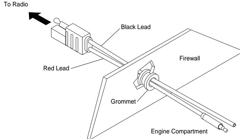
*Figure 2-1. Power Cable Routing into the Engine Compartment*
