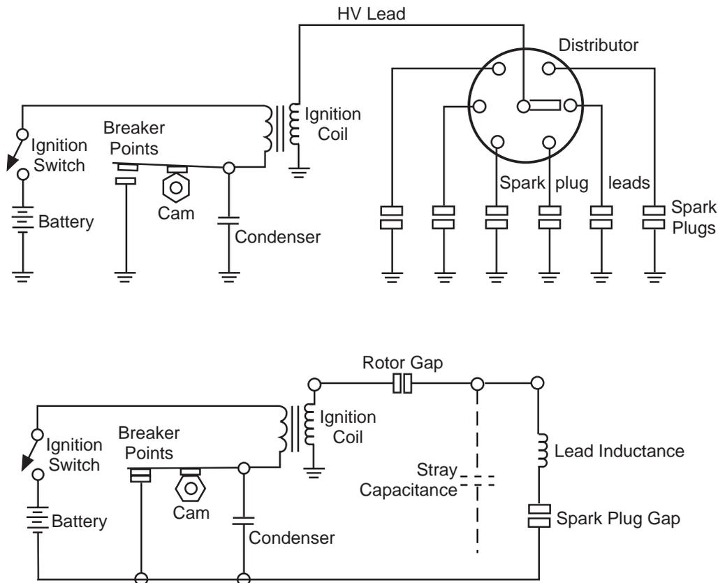
Figure 8-1. Typical Vehicular Ignition System, Simplified Schematic Diagram
