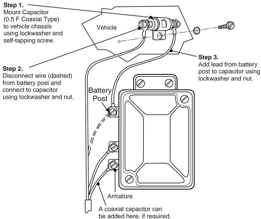
Figure 10-4. Voltage Regulator Noise Suppression
