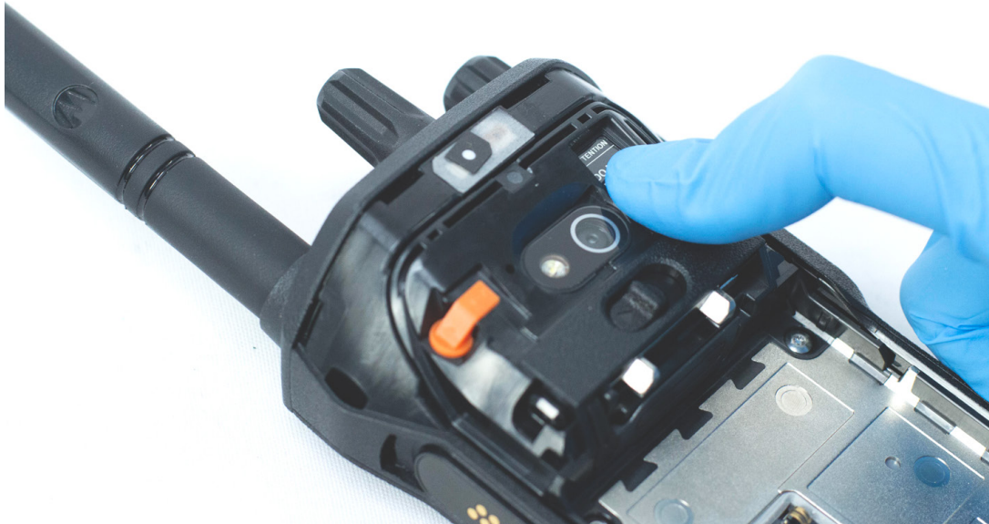
Figure 30: Installing Air Ventilation Label
