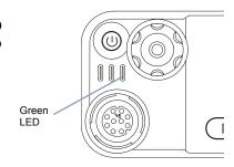
NOTE: The green LED lights up while the radio is transmitting and double blinks rapidly when the radio is receiving a privacy-enabled call.
