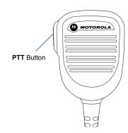
The microphone is activated when the PTT button is pressed.
