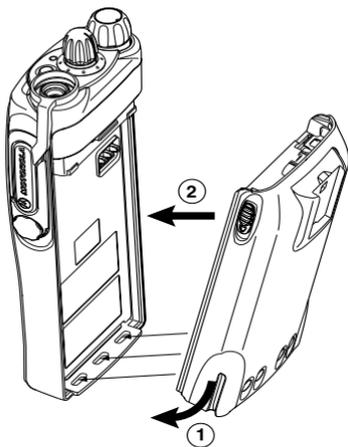
1. Fit the extensions at the bottom of the battery into the slots at the bottom of the radio's body.
