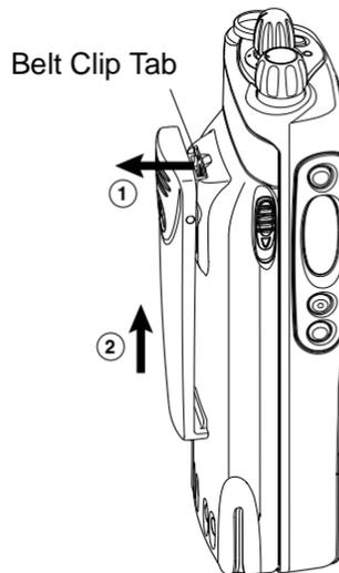
1. Use a key to press the belt clip tab away from the battery.
