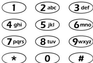
These keys are used when dialling a phone number, making a radio call or entering information for programming the radio's lists.
