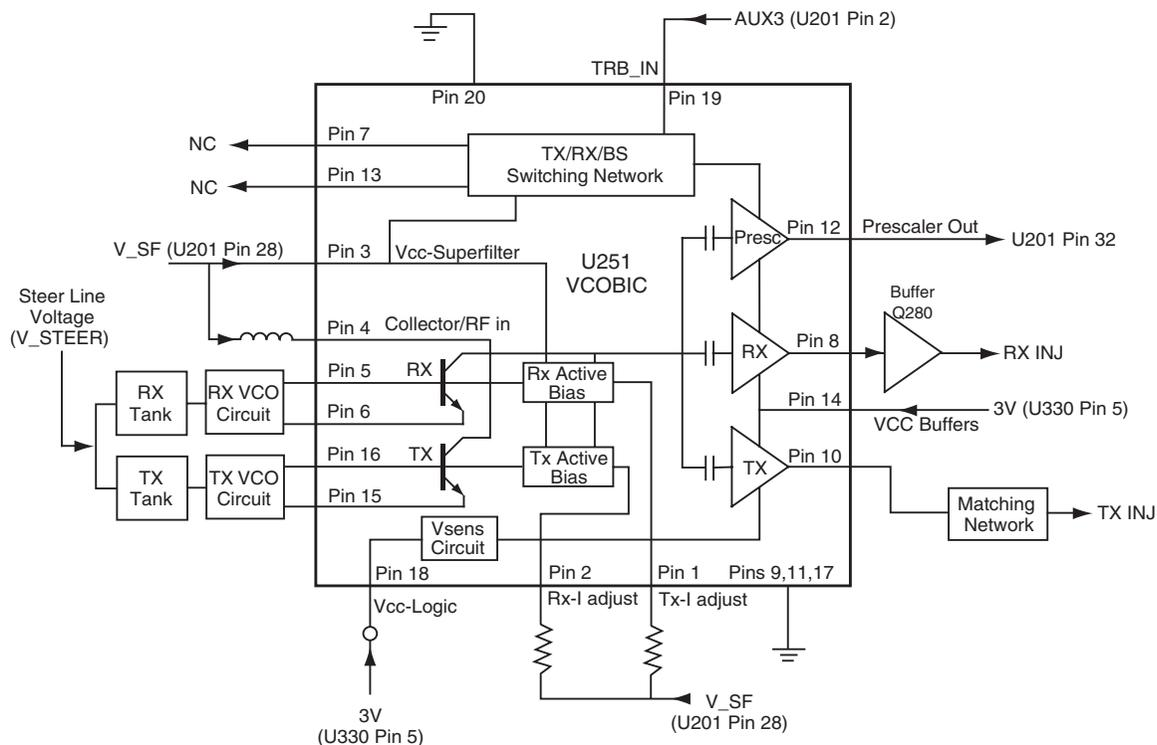
Figure 11-5. UHF VCO Block Diagram
