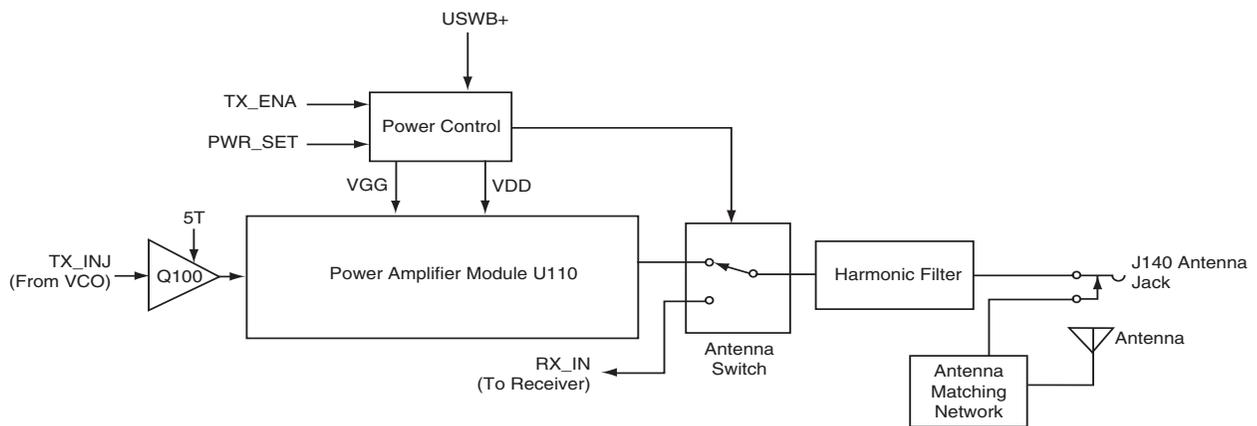
Figure 11-2. UHF Transmitter Block Diagram
