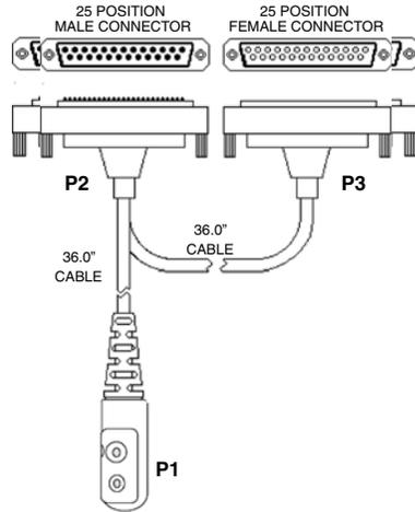
Figure 1-1. Programming/Test Cable
