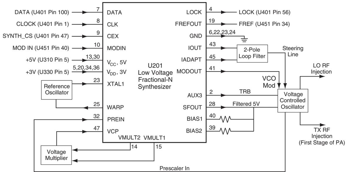
Figure 11-4. UHF Synthesizer Block Diagram
