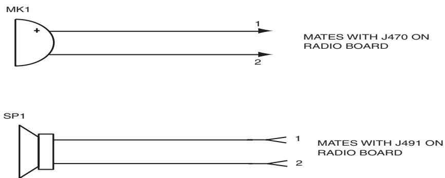
Figure 13-2. Speaker and Microphone Schematic
