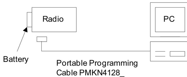
Figure 4-1. CPS Programming Setup
