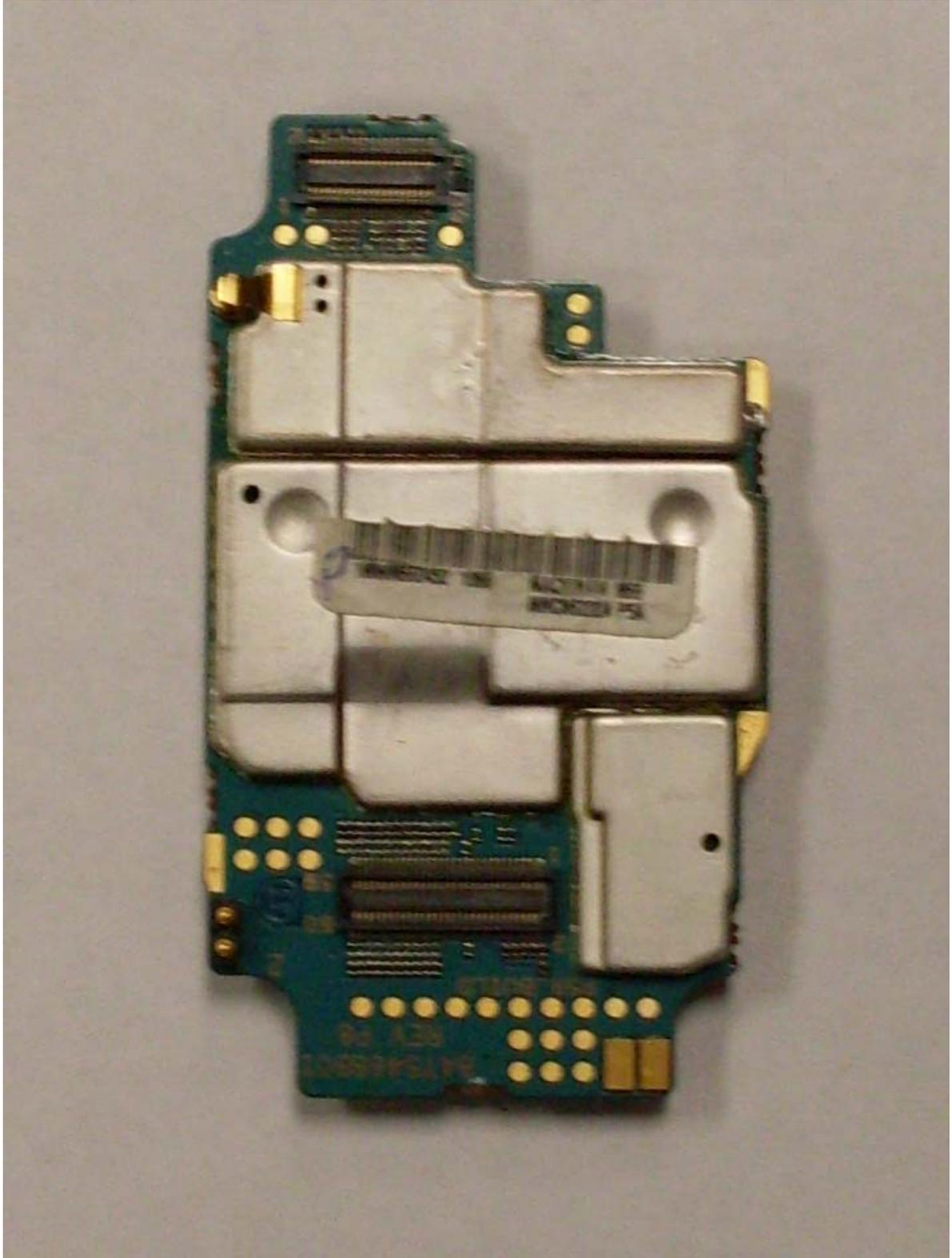
Vocon board with shields board (Bottom)
