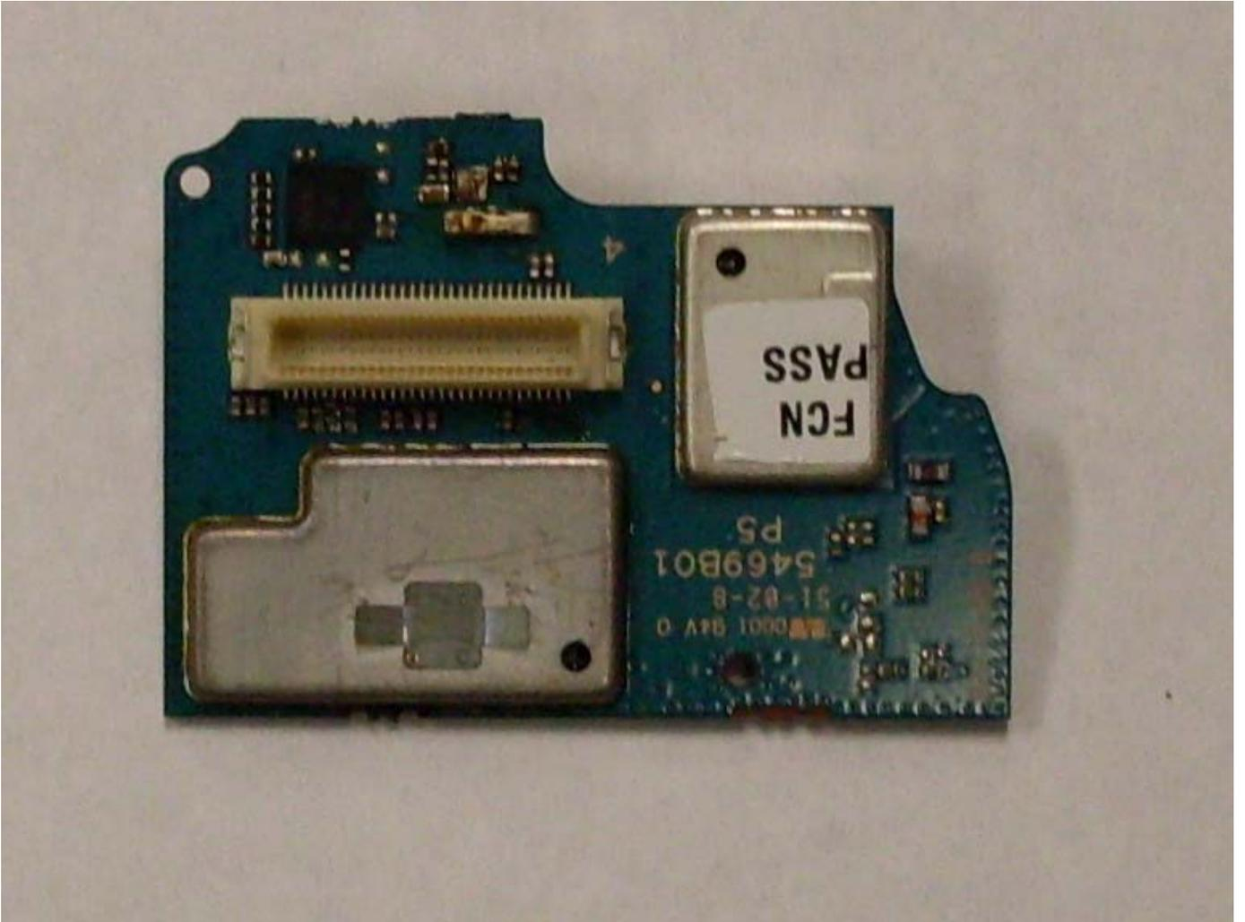
Expander board with shields board (Bottom)
