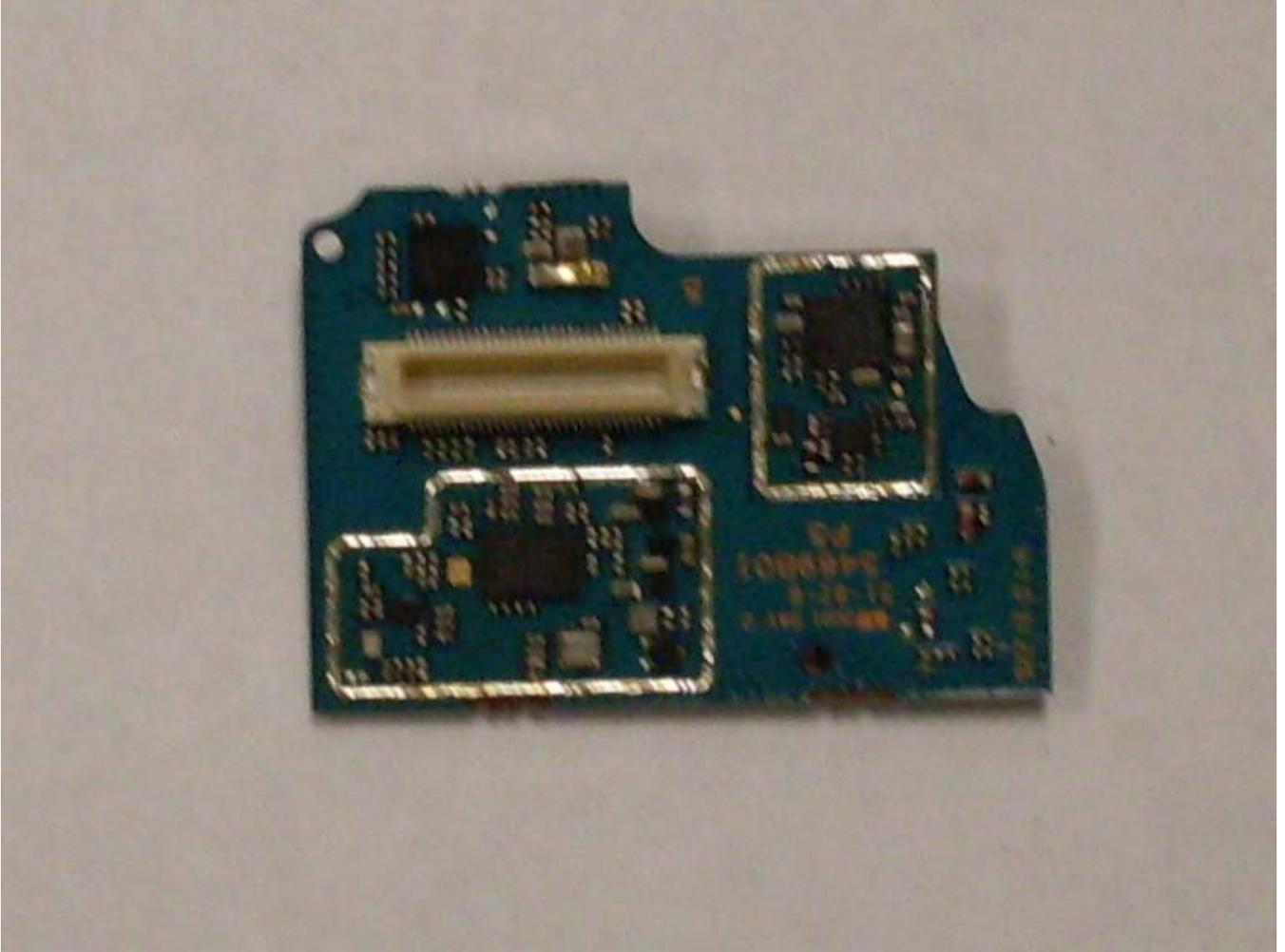
Expander board without shields board (Bottom)
