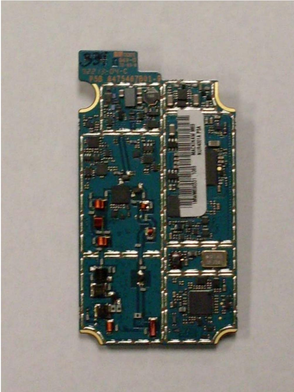
RF board without Shields (Bottom)
