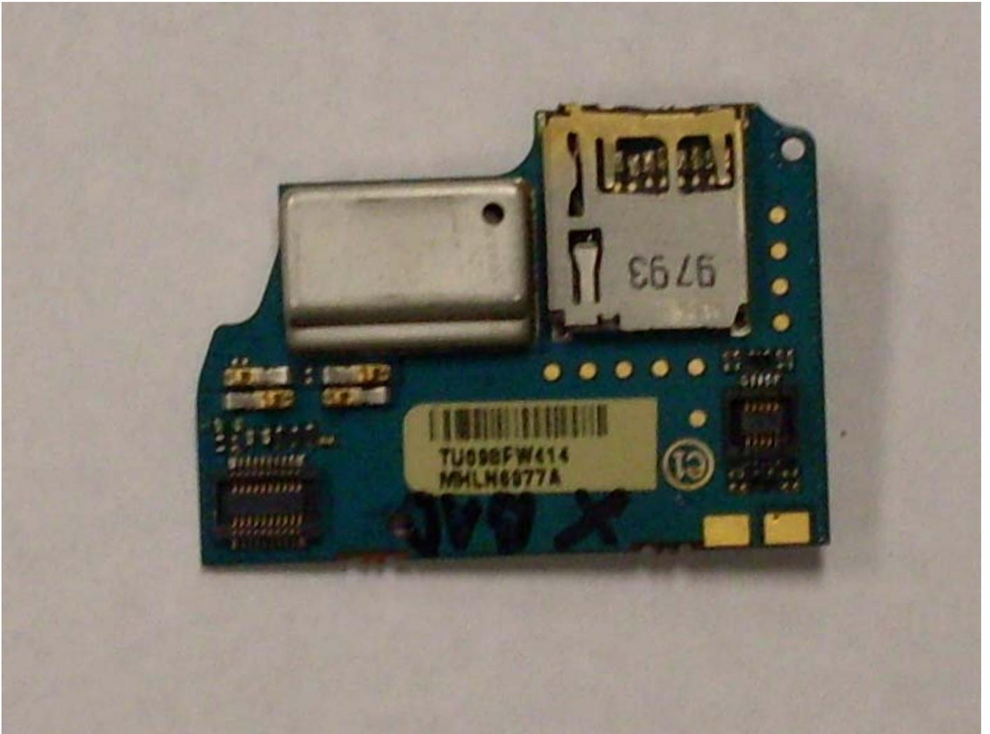
Expander board with shields board (Bottom)
