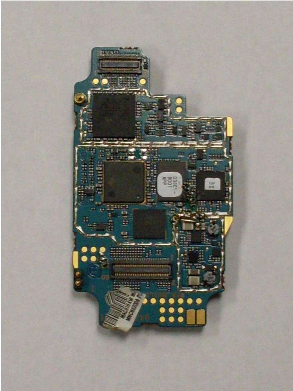
Vocon board without shields board (Bottom)
