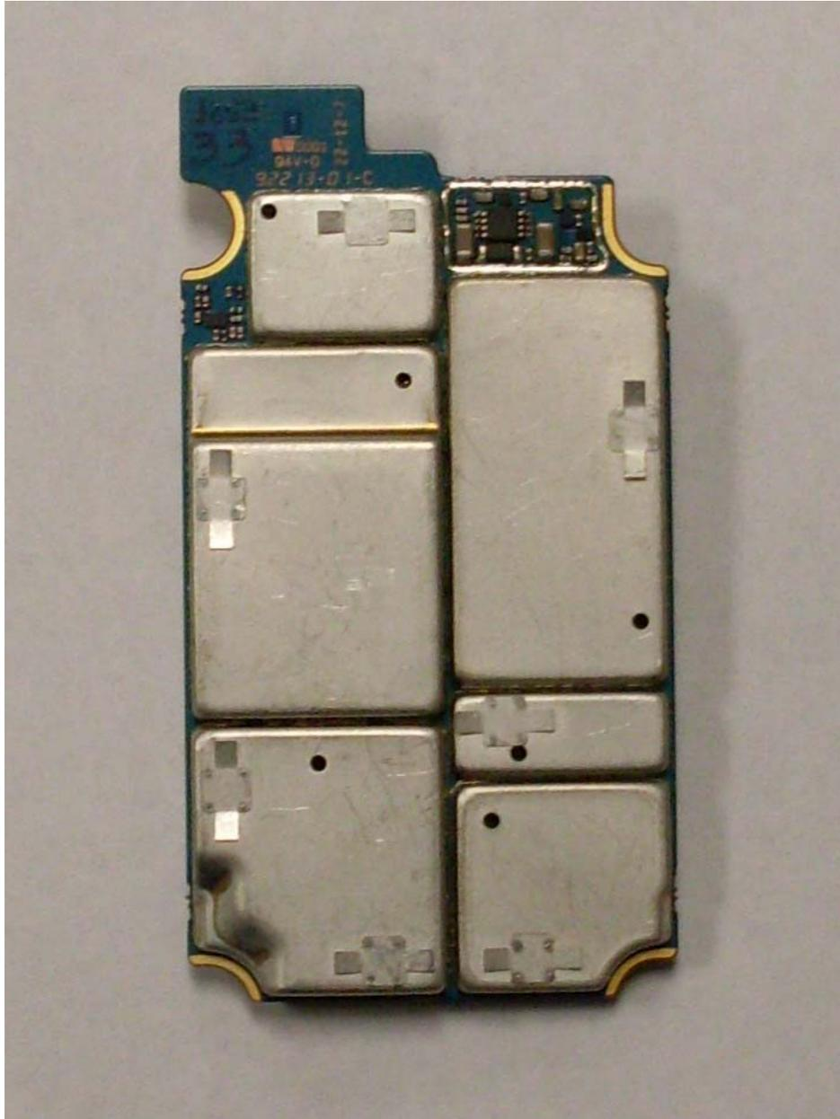
RF board with Shields (Bottom)
