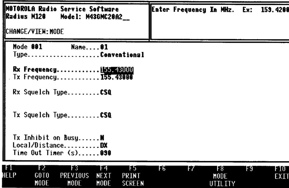
Figure 3-12. Change View, Crossband Transmit Radio Mode
