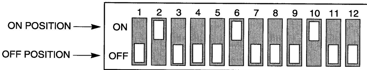
Figure 3-7. S2 Settings for Unidirectional Repeater Using an 8-Channel GM300, M10, or M120 Transmit Radio
