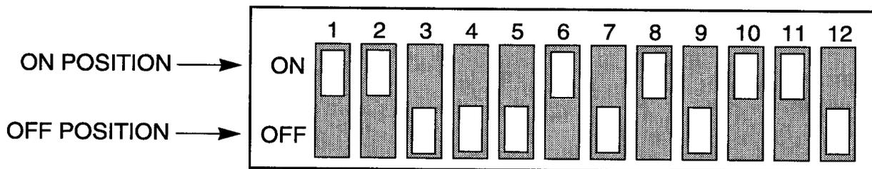
Figure 3-13. S2 Settings for Bidirectional Repeater
