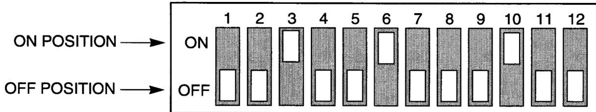
Figure 3-2. S2 Settings for Unidirectional Repeater
