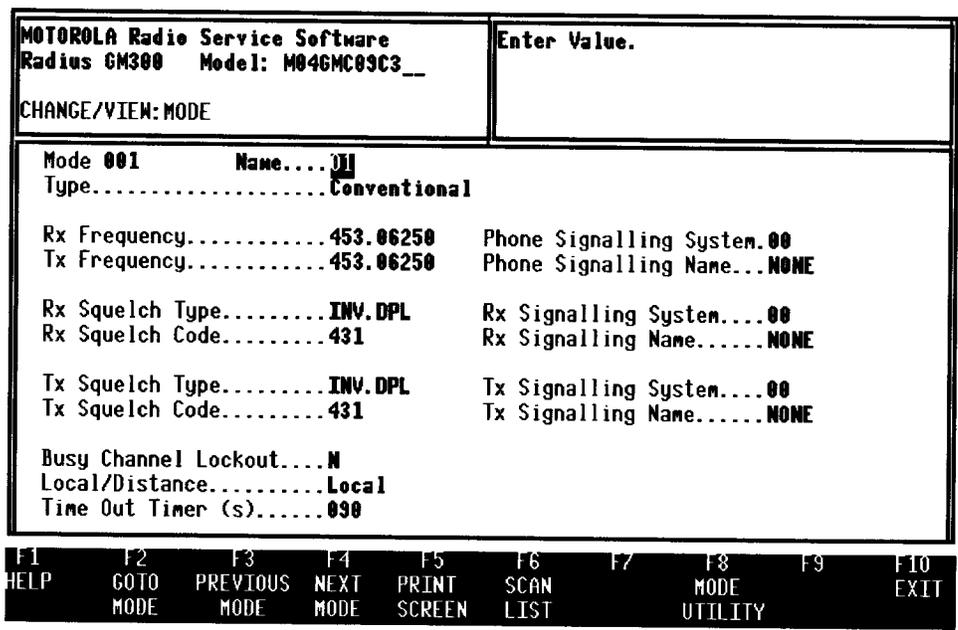
Figure 3-11. Change/View, Crossband Receive Radio Mode
