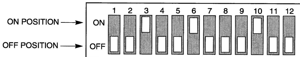
**Figure 3-9.** S2 Settings for Unidirectional Repeater Using an 8-Channel GM300, M10, or M120 Receive Radio
