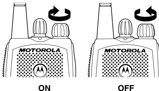
Turn the **On/Off/Volume Control** knob clockwise. If power-up is successful, you will hear the Self-Test Pass Tone (
