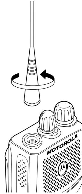
Turn the antenna counter-clockwise to remove it.
