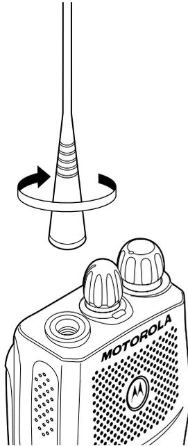
Turn the antenna clockwise to attach it.
