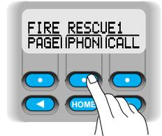
3. The display changes to show the last telephone number dialed or the last ID number transmitted/received. The **[LIST]** softkey also appears.
