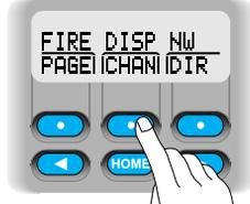
3. The display changes to show the zone name (on steady) and the current channel name (flashing). In the example shown, “FIRE” = Zone, “DISP NW” = Channel.
