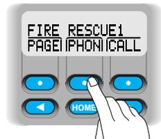
5. The display will show the first member in the list (name on the upper line, number on the lower line). The
