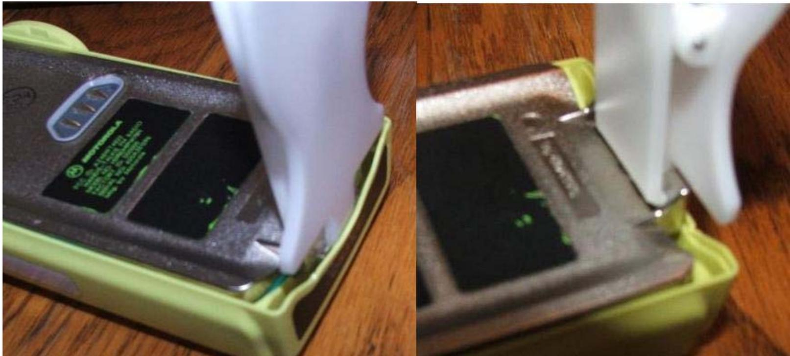
After you get the front shield separated from the chassis, you'll have the radio disassembled to this point (note the o-ring is intact and undamaged):
