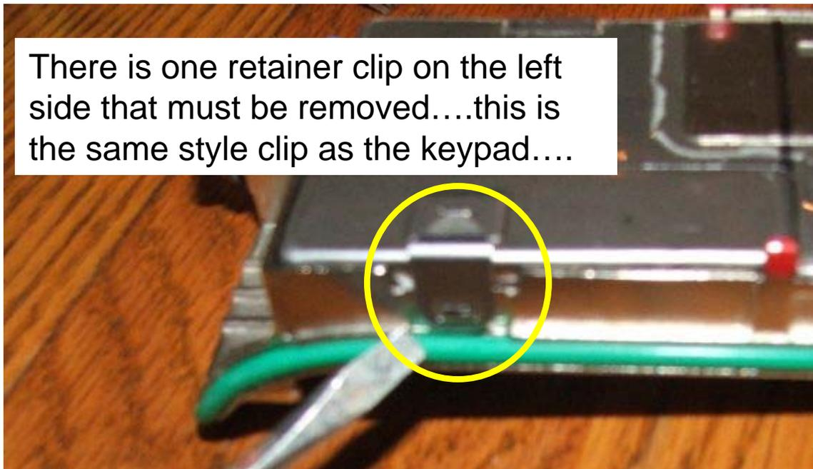
And two detents need to be “popped” on the right hand side to remove the RF shield.....
