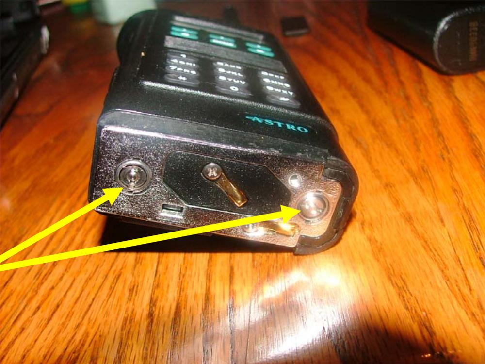
Step 2: Loosen the two slotted screws at the bottom... no need to remove the belt clip....
