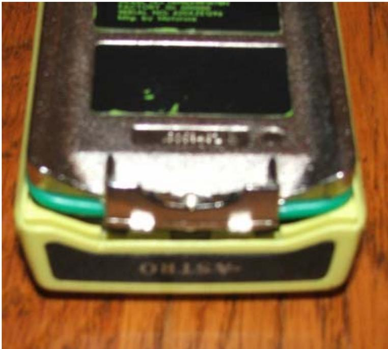
Make sure the o-ring is properly seated along the left and right of the frame and you'll end up with the picture on the left here.... Ready for the final "seat" into the case...
