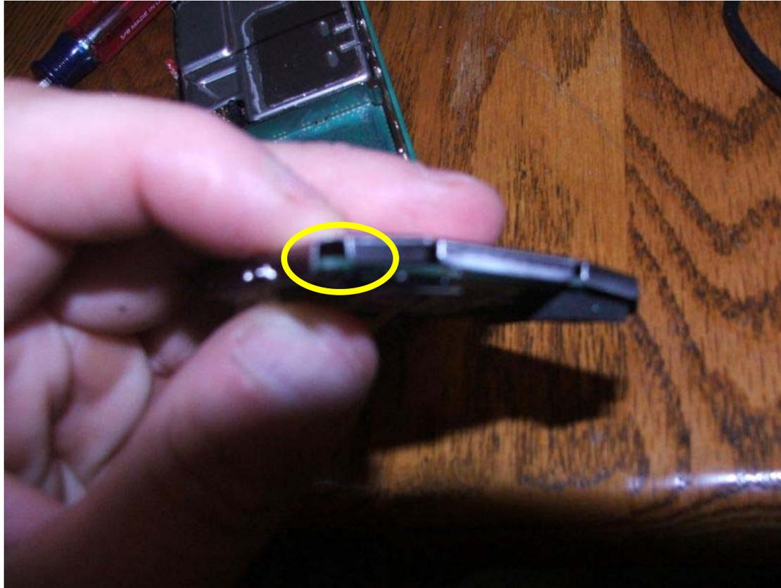
This is a side view of the secure module and it's mounting tray. Note the gap between the secure module and the retainer – THIS IS NOT INSTALLED CORRECTLY and must be fixed before installation....
