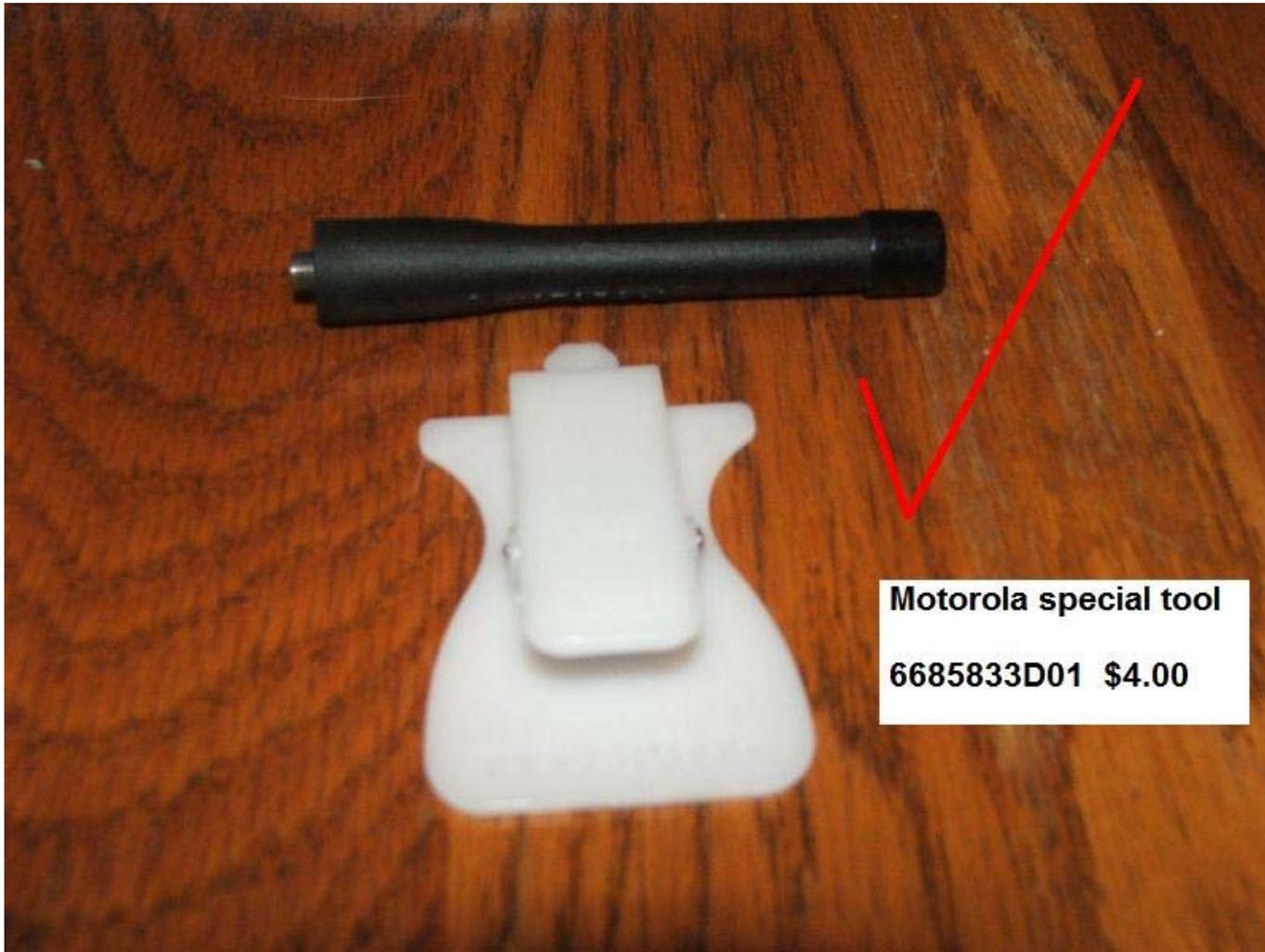
Without this tool, I can guarantee that you will either split the end of the case plastic, as shown in the below picture, or gouge/destroy the protective o-ring.
