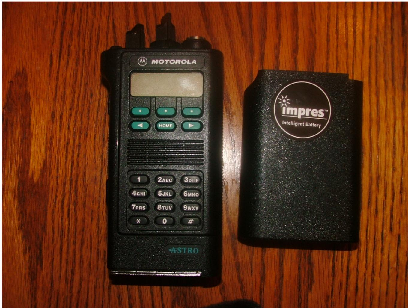
The Astro Digital Saber, Model 3, VHF with the new HNN9033 Impress battery
