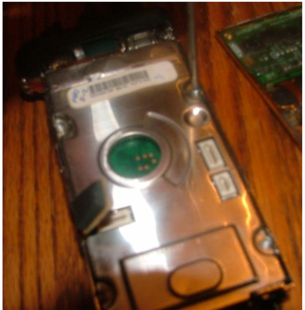
Now the fun part. You have to remove four little phillips screws to get the vocon out of the chassis. These are very easy to strip the screwheads out of – so please be careful and use a proper fitting screwdriver.... They are also easily lost – so put them in a plastic cup! It's very common to find used radios missing one or two of these screws!
