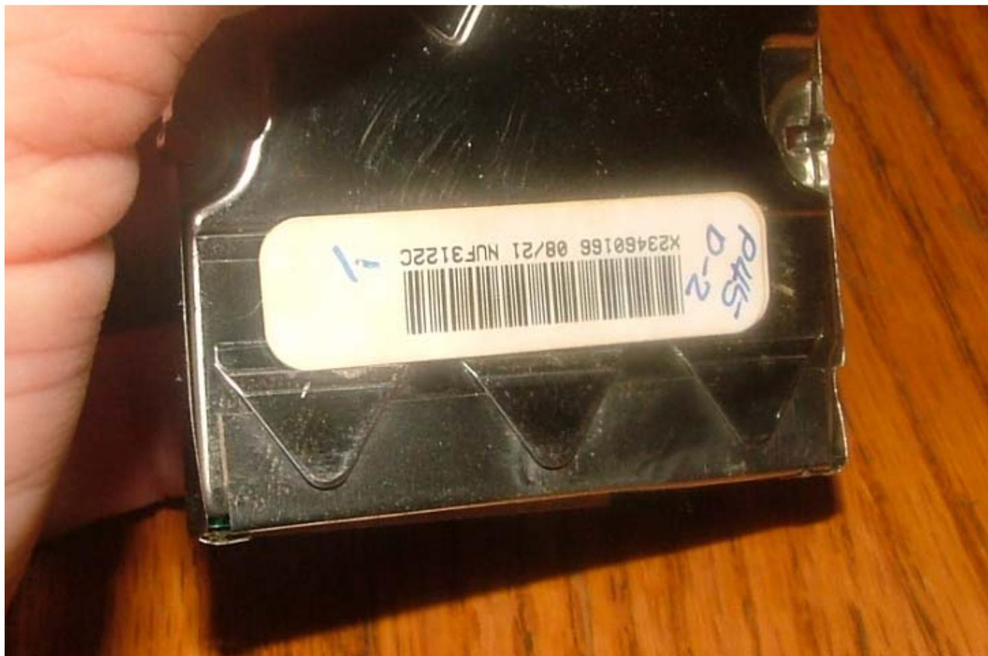
Pay attention how the two halves of the vocon shield fit together.
