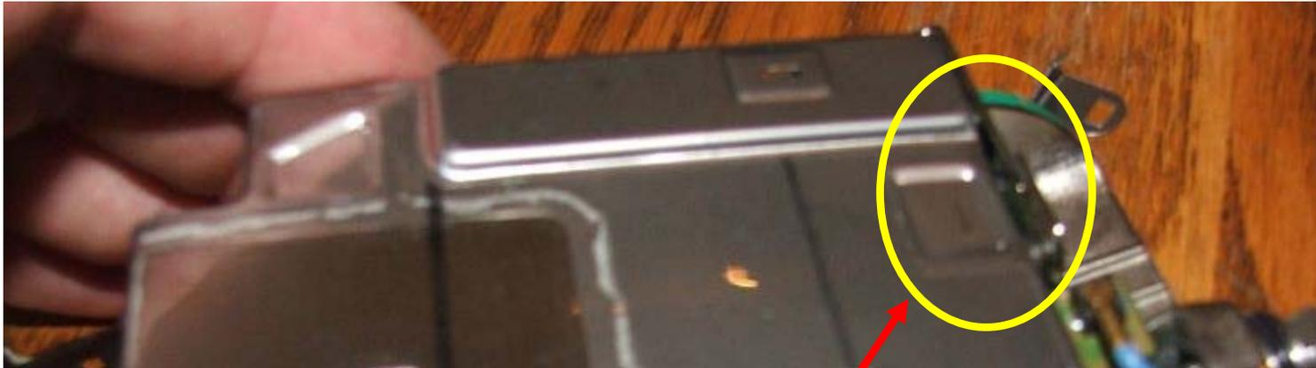
There are two small detents that must be disengaged to remove the RF board shield. Note the **blue** RF cable – be VERY careful with this cable – it's two ended – and connects the RF board to the antenna connector – it's VERY EASILY damaged.
