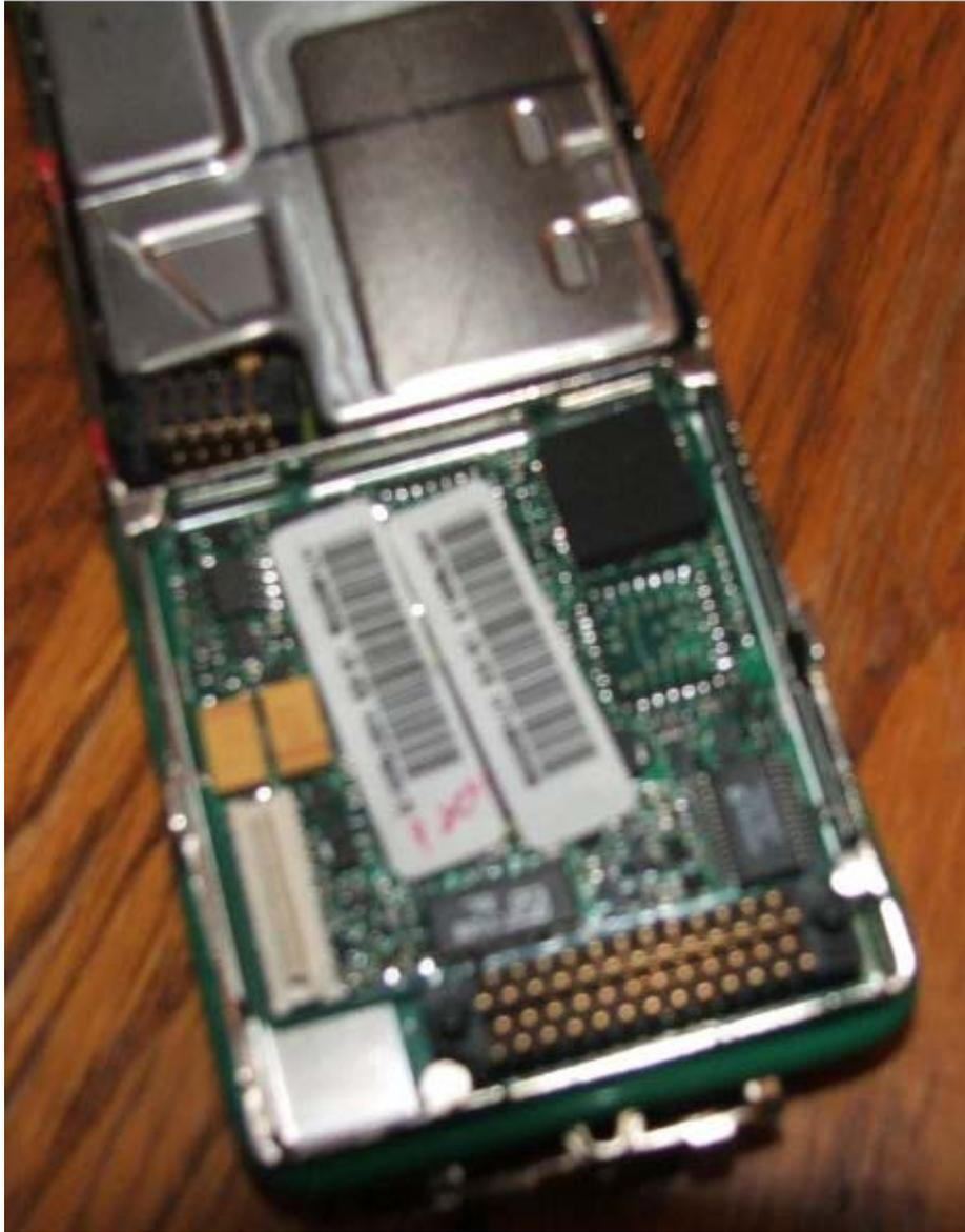
One properly installed secure module... note that the metal secure module retainer board is snug against the chassis....
