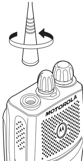
Turn the antenna counter-clockwise to remove it.
