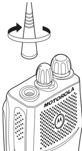
Turn the antenna clockwise to attach it.
