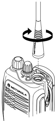
Turn the antenna clockwise to attach it.
