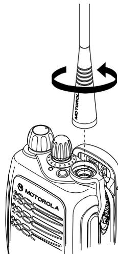
Turn the antenna counterclockwise to remove it.
