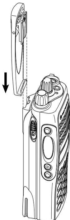
1. Align the grooves of the belt clip with those of the battery.
