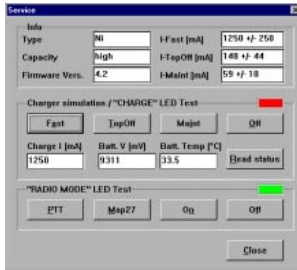
Figure 2-4 Vehicle Adapter Service Screen
