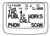
This figure is typical of what you see on your radio. The 64 x 96 pixel liquid crystal display (LCD) shows radio status, text, and menu entries.
