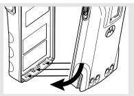
2 Press both sides at the top of the battery against the radio until both latches click into place.
