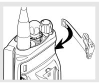
2 Snap the larger end of the adapter into place in the shroud indent, below the antenna port.
