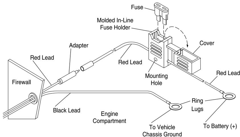
**Figure 1-2** Power Cable Assembly
