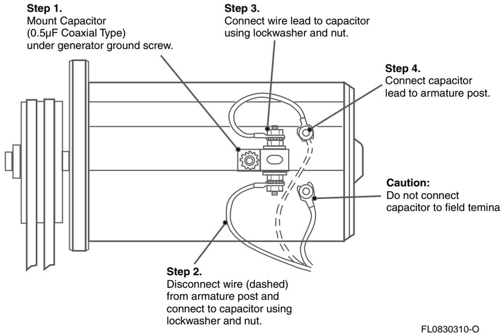
**Figure 2-6** Generator Whine Suppression
