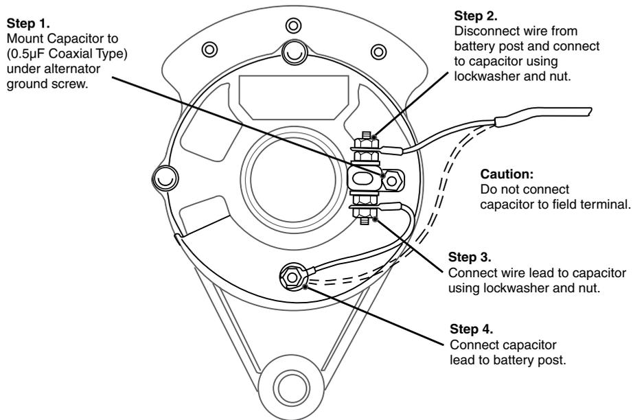
**Figure 2-7** Alternator Whine Suppression
