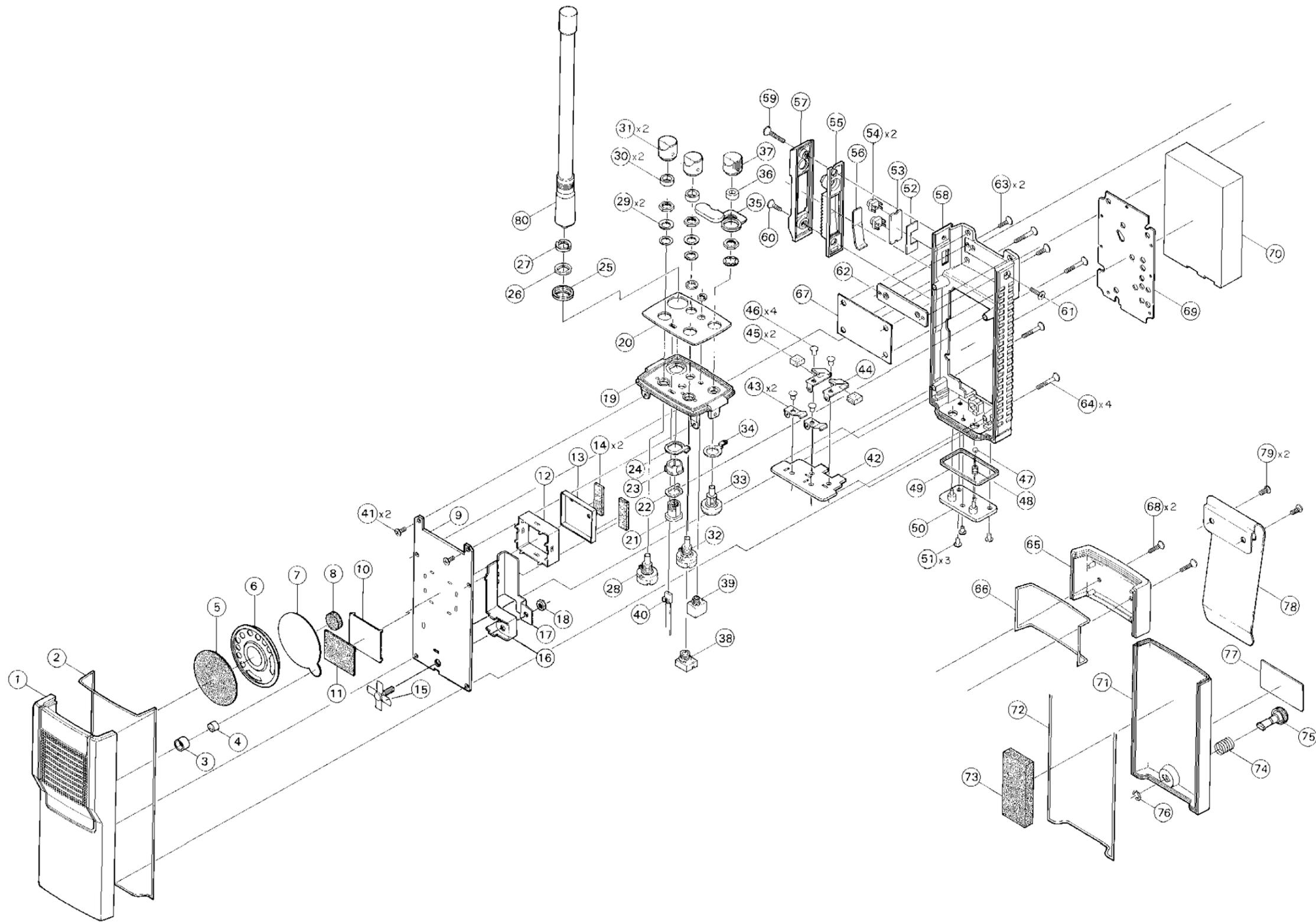
Radio Assembly, Exploded View
