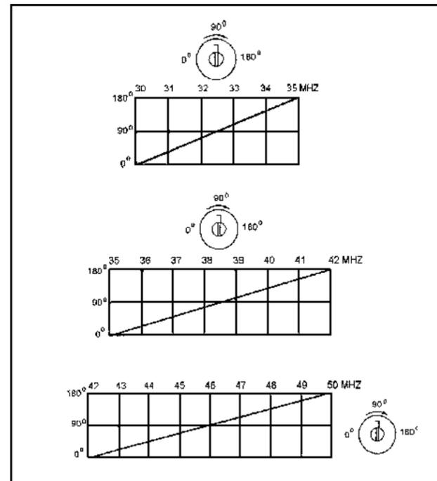
Figure 5 - Antenna Tuning Capacitor Settings Vs Frequencies
